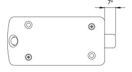
CAN BE MOUNTED USING THE SELF ADHESIVE PAD PROVIDED OR SCREW MOUNTED VIA 2x
