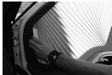
C5: Bring handle up to stop rail, magnetic catch locks automatically.
