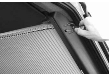
B22: Pull the blind closed. The gap between the blind and the instrument panel or the roof can be adjusted by rotating the fixing screws.
