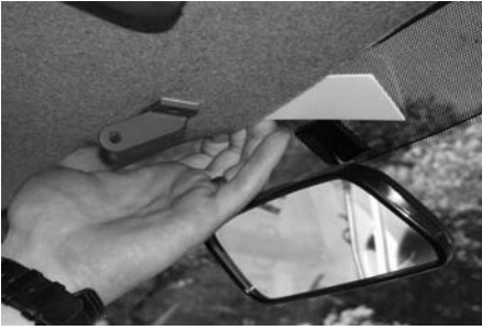
B16: Push plastic strip behind the roof covering.
