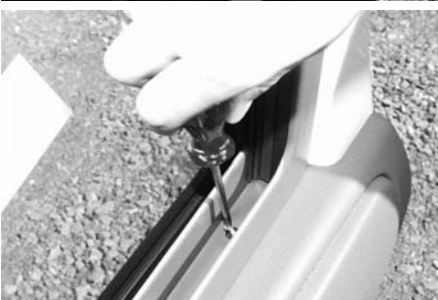
B26: Insert frame and screw. (Screws LIK3.5x16)
