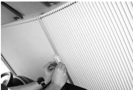
C3: Bring handles together in the middle, magnetic catch locks blinds automatically.
