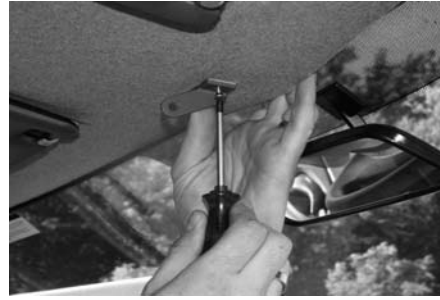
B17: Hold plastic strip and carrier while screwing on. (Screws SK4.2x13)
