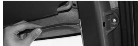
B20 & B21: Repeat procedure for top guide tube.
