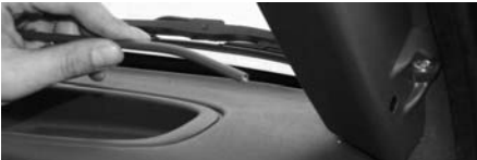
B18 & B19: Push the bottom guide tube through the carrier on the instrument panel and fix with the screws in the left and right cassettes.
