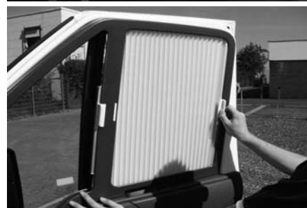
C7: Bring handle up to stop rail, magnetic catch locks automatically.
